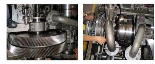
Modified Gear ratio retrofitted in existing hydraulic coupling
